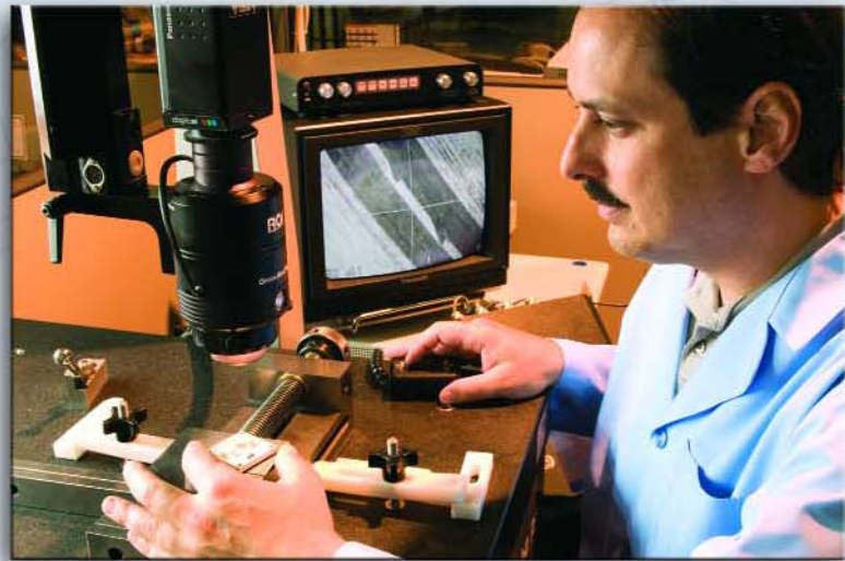
Advanced coordinate measurement instruments seek out minute flaws that could hamper pump performance.
